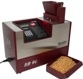
A red and silver electronic device with a digital display and a small tray of pecans next to it. | SB900                      | Secondary methods were developed wherein the electrical properties of pecans can be measured and converted into moisture content. |
